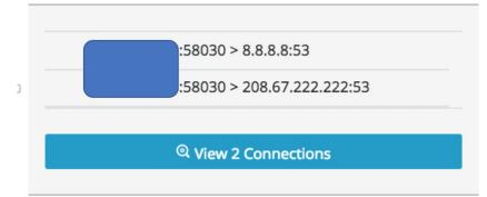
The screenshot below shows the traffic generated by the backdoor and demonstrates DNS Tunneling for C2 communication. As shown, while the destination IP is "8.8.8.8" – Google's DNS server – the malicious domain is "hiding" inside the DNS packet:
