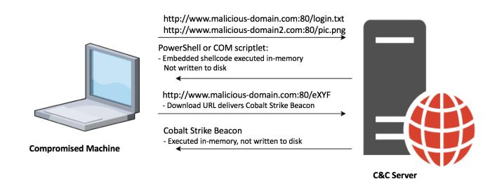
In the first phase of the attack, the attackers used a fileless in-memory payload delivery infrastructure consisting of the following components:
